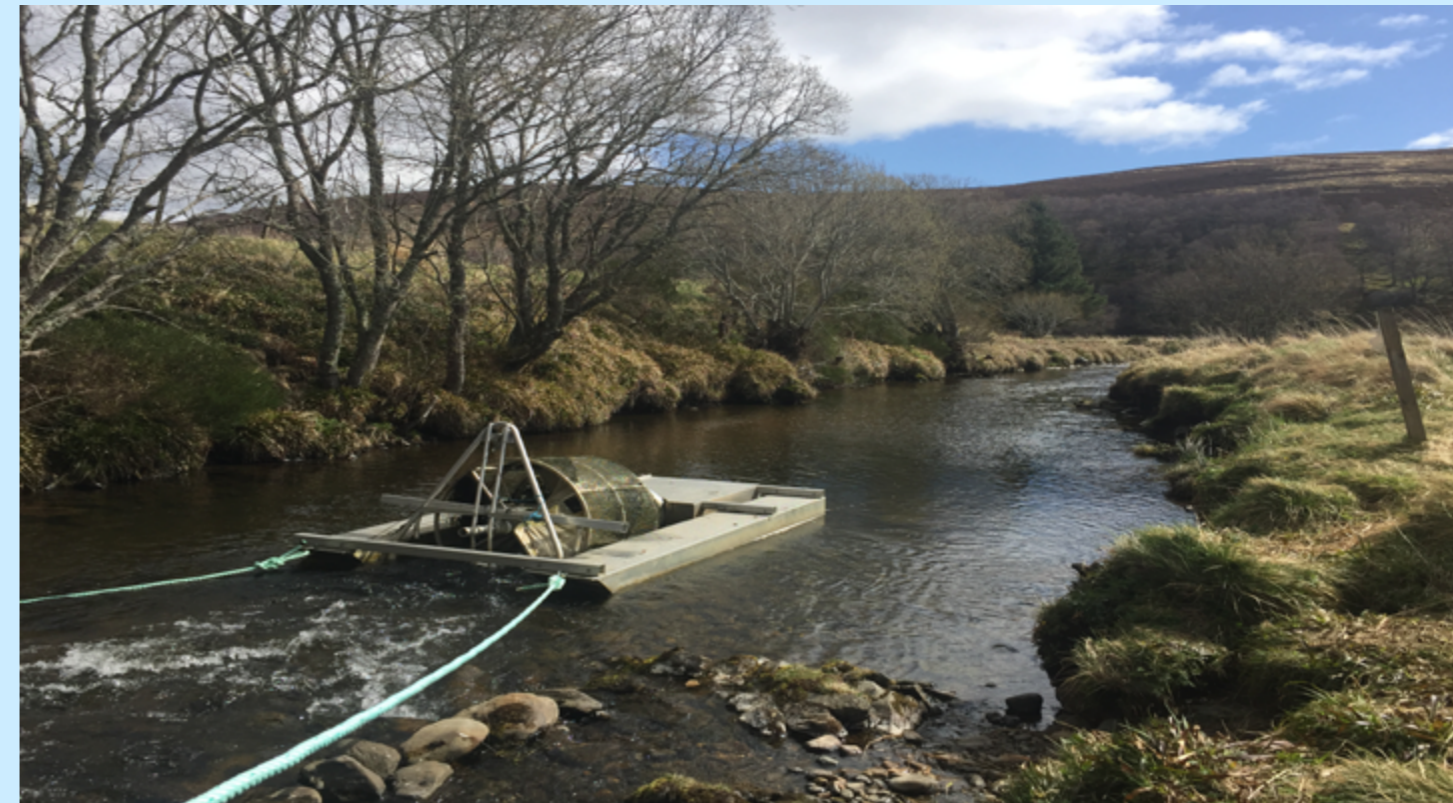
Rotary screw trap. ©Atlantic Salmon Trust
