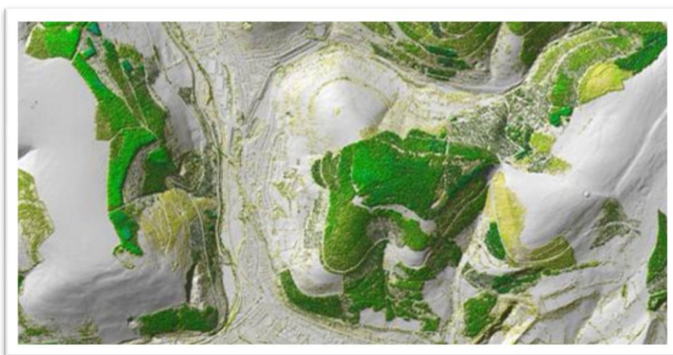
Figure 7. Part of JPEG image of LiDAR derived vegetation object map showing vegetation over 2.5m
