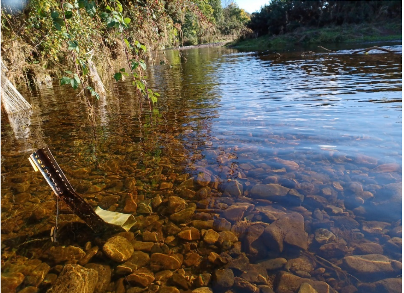
Figure 2. Picture illustrating how temperature loggers are placed in river. The temperature logger is covered with white plastic sheath to block the sun from heating the logger up further, allowing for only water temperature to be recorded.
