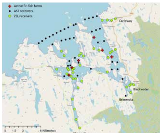
The acoustic receiver array deployed in Loch Roag and associated rivers.
