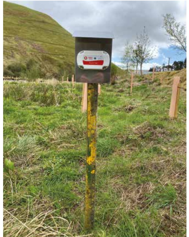
Remote land-based temperature sensor to monitor changes in air temperature as the habitat scheme matures
